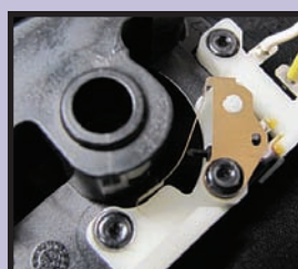
Heatstaking Multiple points and planes
