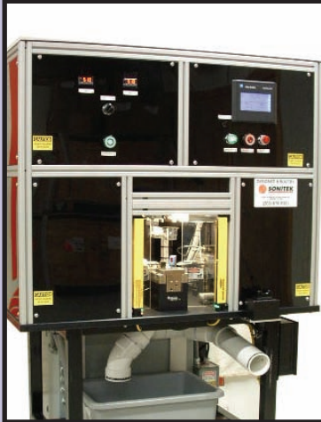
Custom designed heatstaking system.
