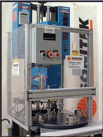
4-Station Rotary with Auto-eject
