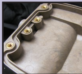
Insertion Install 1 or 100+ inserts
