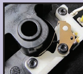
Heatstaking Multiple points and planes
