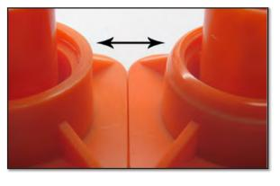
Swage walls of plastic to entrap metal objects or other foreign objects like PCB's and encase them into your plastic parts.
