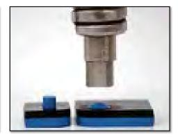
Staking is the process of connecting two components by creating an interference fit between the two pieces. One workpiece has a hole in it while the other has a boss that fits within the hole. The boss is very slightly undersized so that it forms a slip fit.
