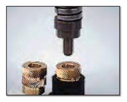
Install metal inserts or fasteners into your plastic housings. Simultaneously install 1 or 100 at a time including onto multiple planes.
