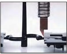
Cut or Trim runners and gates cleanly from your plastic parts and injection molded parts. Degate with vestiges with tight tolerances.
