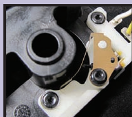
Heatstaking Multiple points and planes
