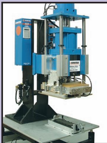
5 Ton Press for Heatstaking
