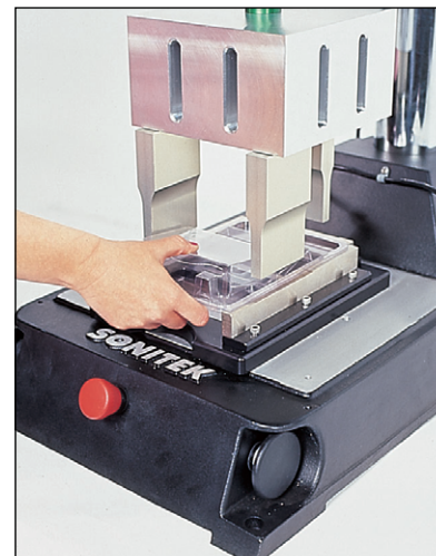
Auto-cycle available, (no pressing of palm buttons) just insert package and machine cycles automatically.
