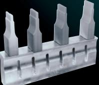
Fig. 5 Large rectangular horn with four extenders
